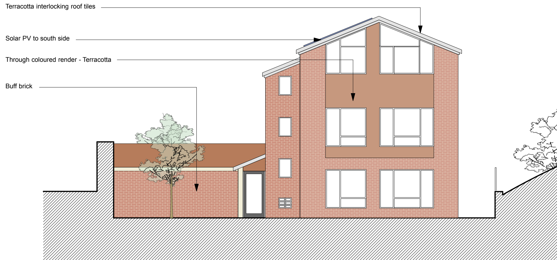
Front (North-West) Elevation
